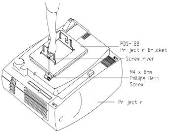
Using a screwdriver, secure the PDS-022 mounting bracket using three (3)
